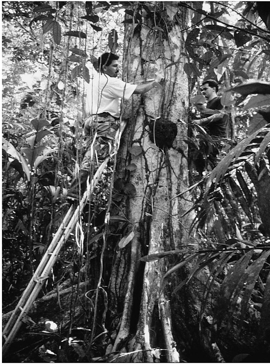
Figure 2. Multiple ladders are required for accurate diameter measurements of many trees in tropical forest inventory plots, both to obtain the diameter of the cylindrical bole at a permanent point of measurement above buttresses and other stem irregularities, and to avoid including vines, termite trails and other objects frequently occurring on tree boles.
